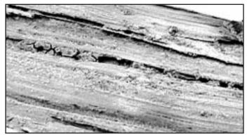
Figure 4. Wood damage caused by Formosan subterranean termites.
